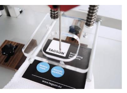
The Tagson PS-1 allows packaging of various types and socks thicknesses. By changing the module you can pack socks **from 7 mm up to 80 mm**. By choosing the correct needle you can pack the finest materials **leaving no damage to the socks**.
