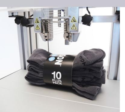
NEW innovative automated hosiery machine for tagging socks up to 100 mm (3,93 inch) in thickness.
